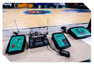
It is also important that the timer pays attention to the flashing of the transmitter LEDs. If the transmitter LEDs are flashing it means the transmitter on the referee's belt is not working properly, or is about to stop working. It is important to advise the relevant referee as soon as possible, during the next dead ball opportunity, so that the transmitter can be changed.
