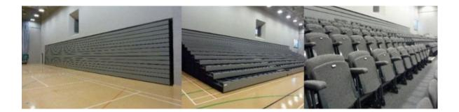
This type of seating will fold away into a recess that is approx. 1.3m deep depending on tread. It can be up to 18 rows without access from the top. Access from the top will increase capacity.
