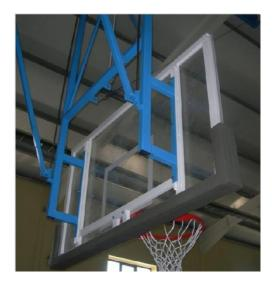
Backboards shall measure 1,800 mm horizontally and 1,050 mm vertically. Backboards can be made of timber or transparent material with a minimum thickness of 19mm
